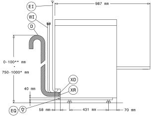
Drain ΕI Electrical inlet (power) EO **Electrical Outlet** HWI Hot water inlet
